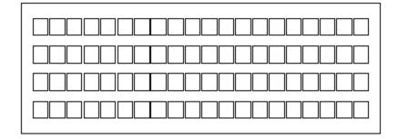
The memory map is always the same regardless of the display configuration, but in this drawing I have shown a small space between addresses 13h and 14h on the first line and another between addresses 53h and 54h on the second line.
